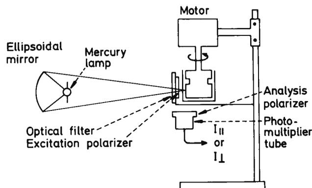
Figure 1: Schematic diagram of Couette viscometer for fluorescence polarization measurements.
